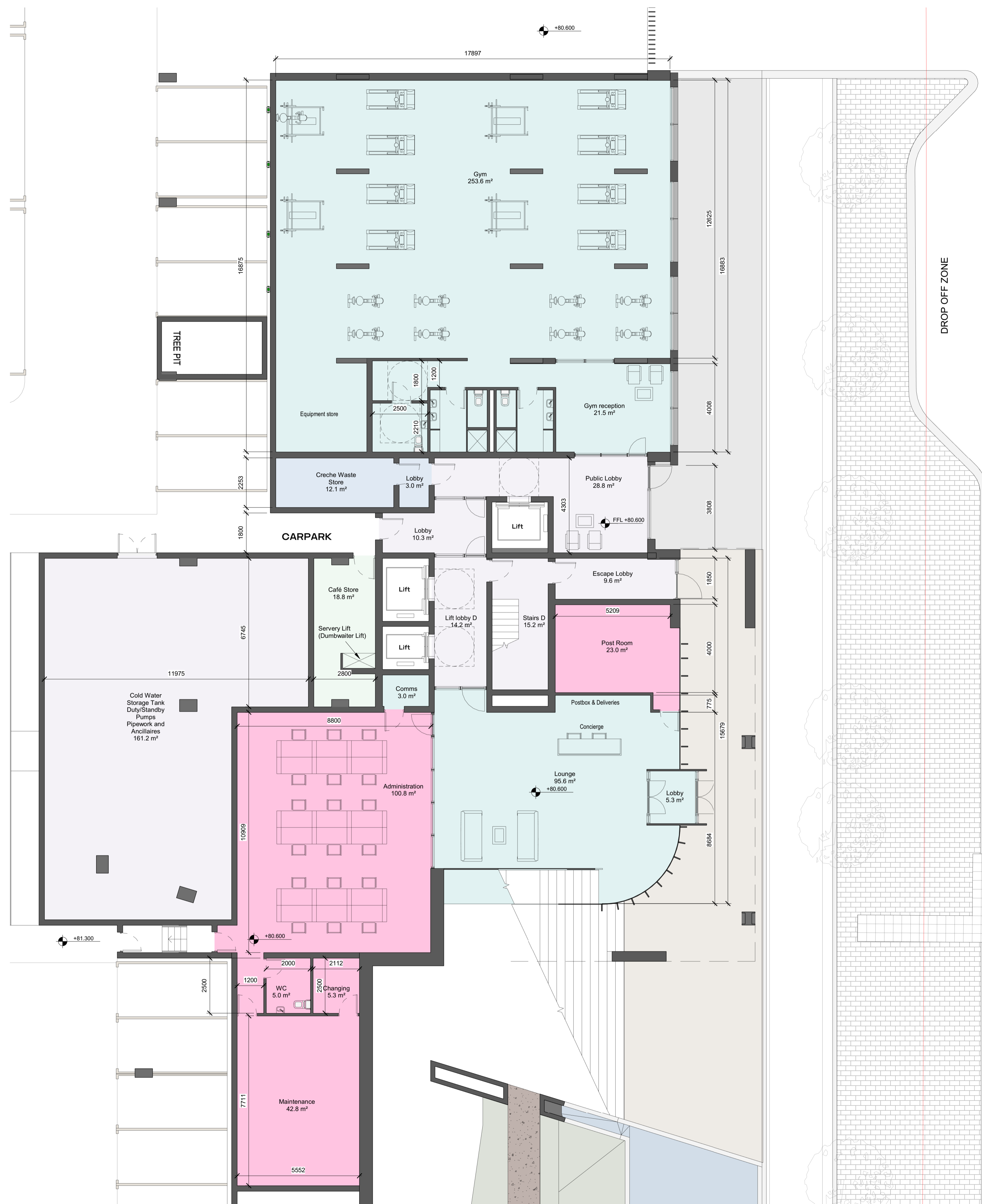
① Block D Amenities Level 0 (Lower Ground Floor Plan) 1:100
